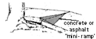
**Figure 11.** A "mini-ramp" can be used to smooth the uneven surface caused by root damage to pavement.
