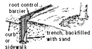
**Figure 12.** A vertical underground barrier will help keep tree roots from damaging concrete as they grow.
